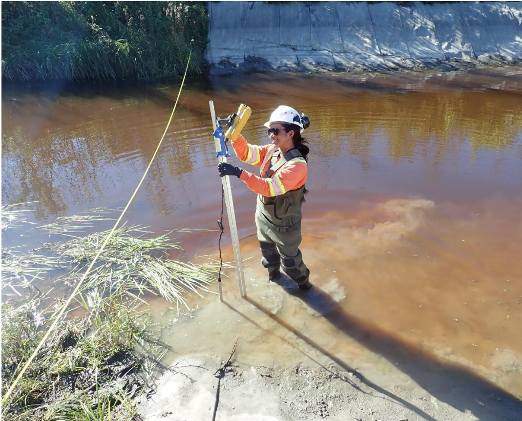
Figure 21. Technician taking flow measurements on the Pinewood River, Fall 2024
