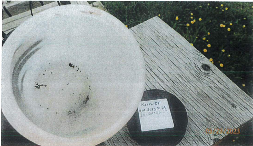
Figure 5: North Station Dustfall jar after sampling during the month of June, 2023, before shipping to certified laboratory.
