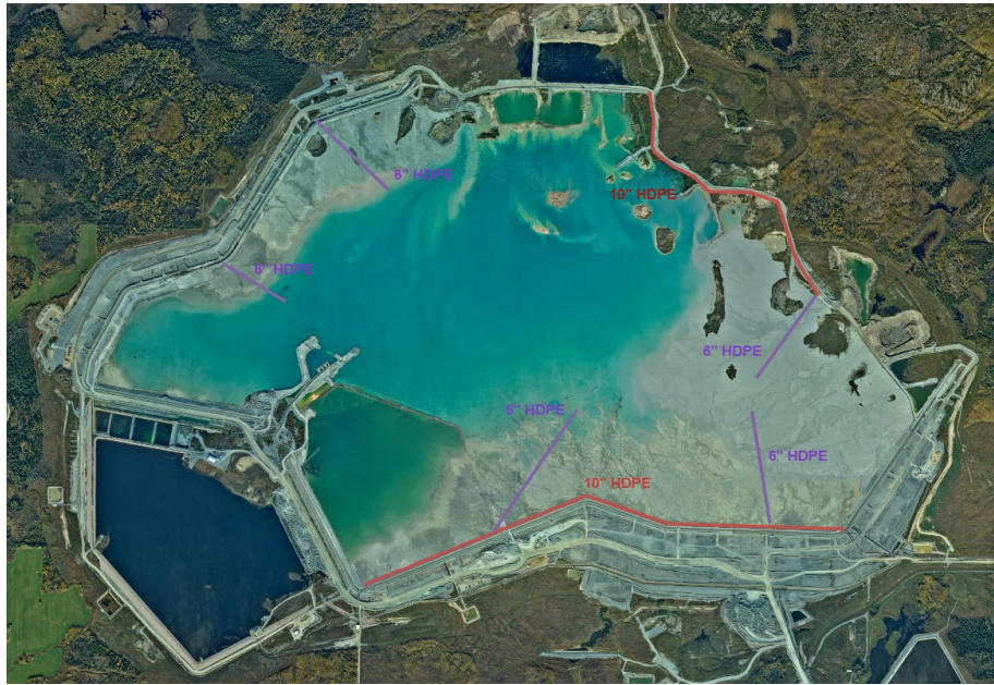
Figure 4: Theoretical layout of TMA perforated piping network planned to be operating by October 2024.
