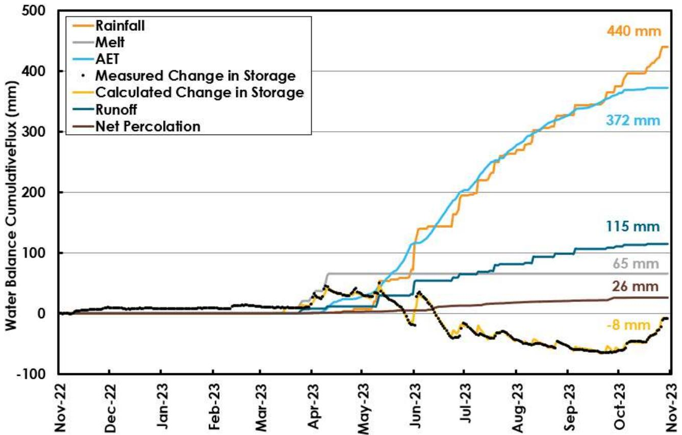
**Figure 3.17 :** Cumulative water balance flux at Trial #1 for the monitoring period.
