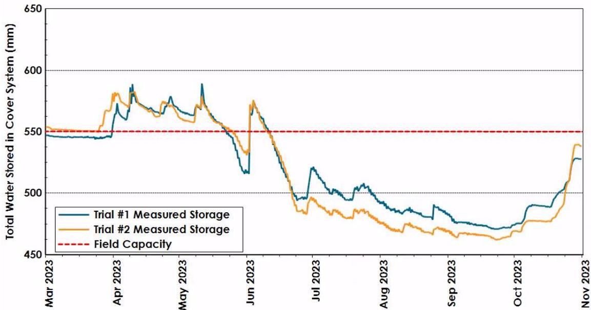
Figure 3.16: Measured storage versus cover system field capacity.
