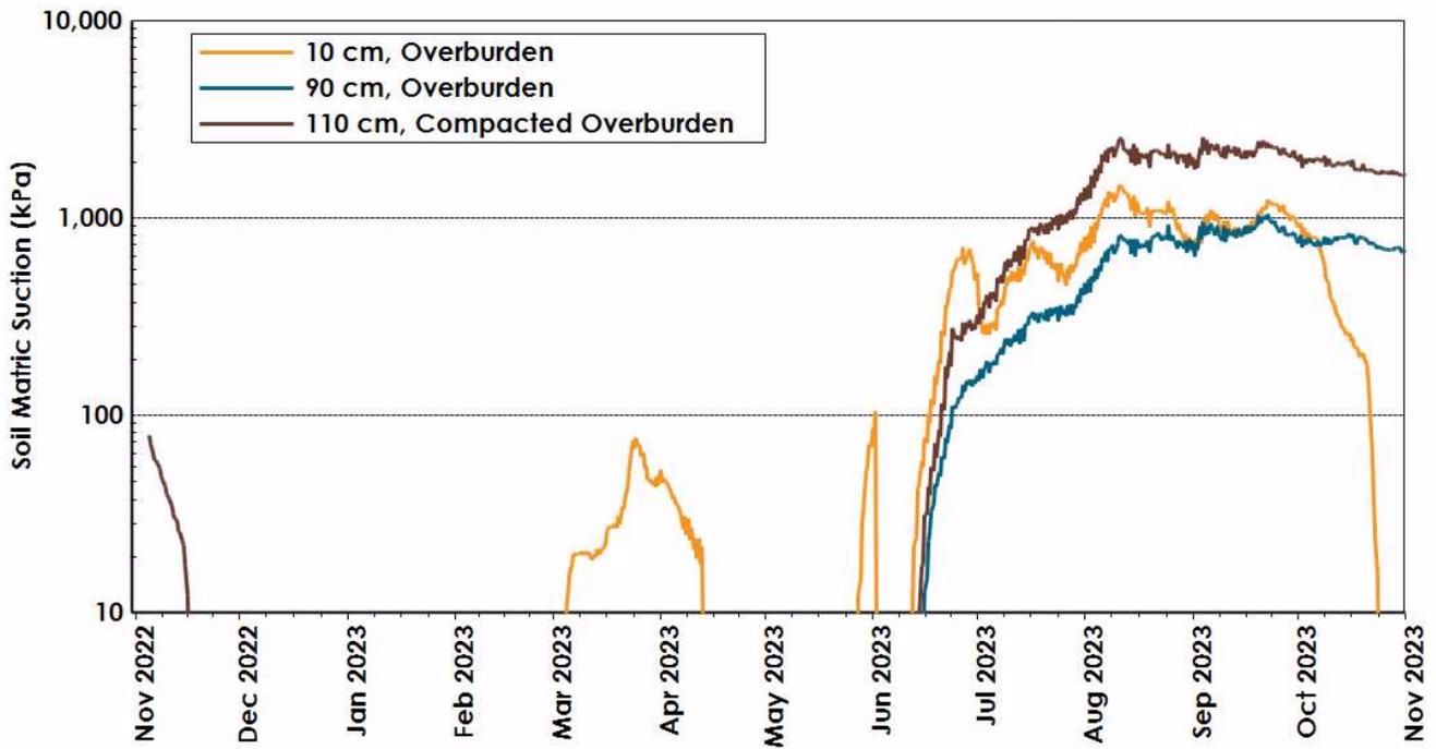
Figure B.8: Suction profile at the Trial #2 secondary station during the monitoring period.
