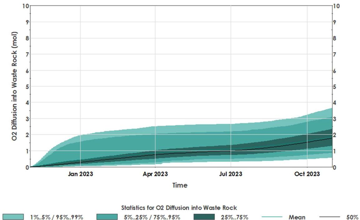
Figure 3.19: Oxygen diffusion simulation through cover materials on Trial #1 over the monitoring period.
