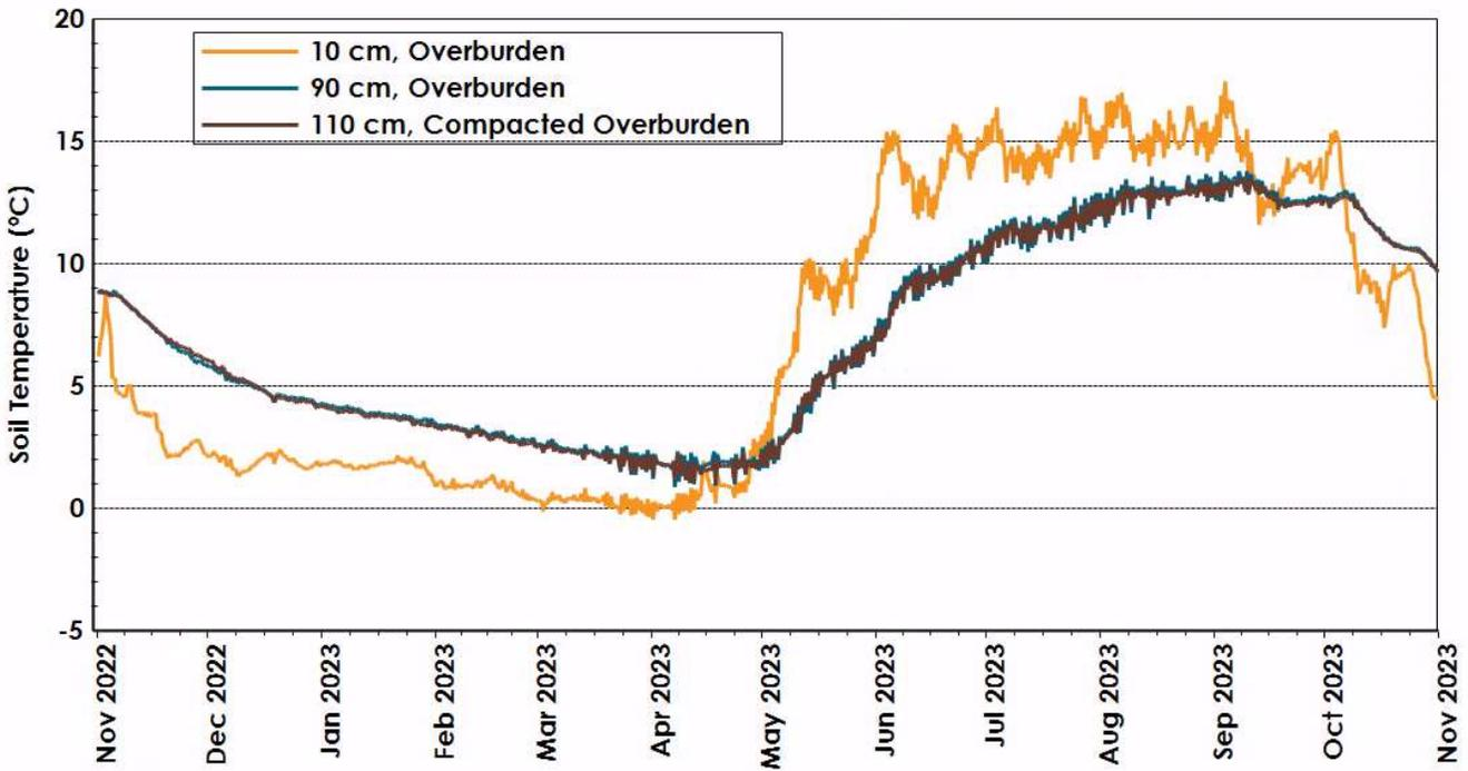
Figure B.10: Temperature profile at the Trial #1 secondary station during the monitoring period.
