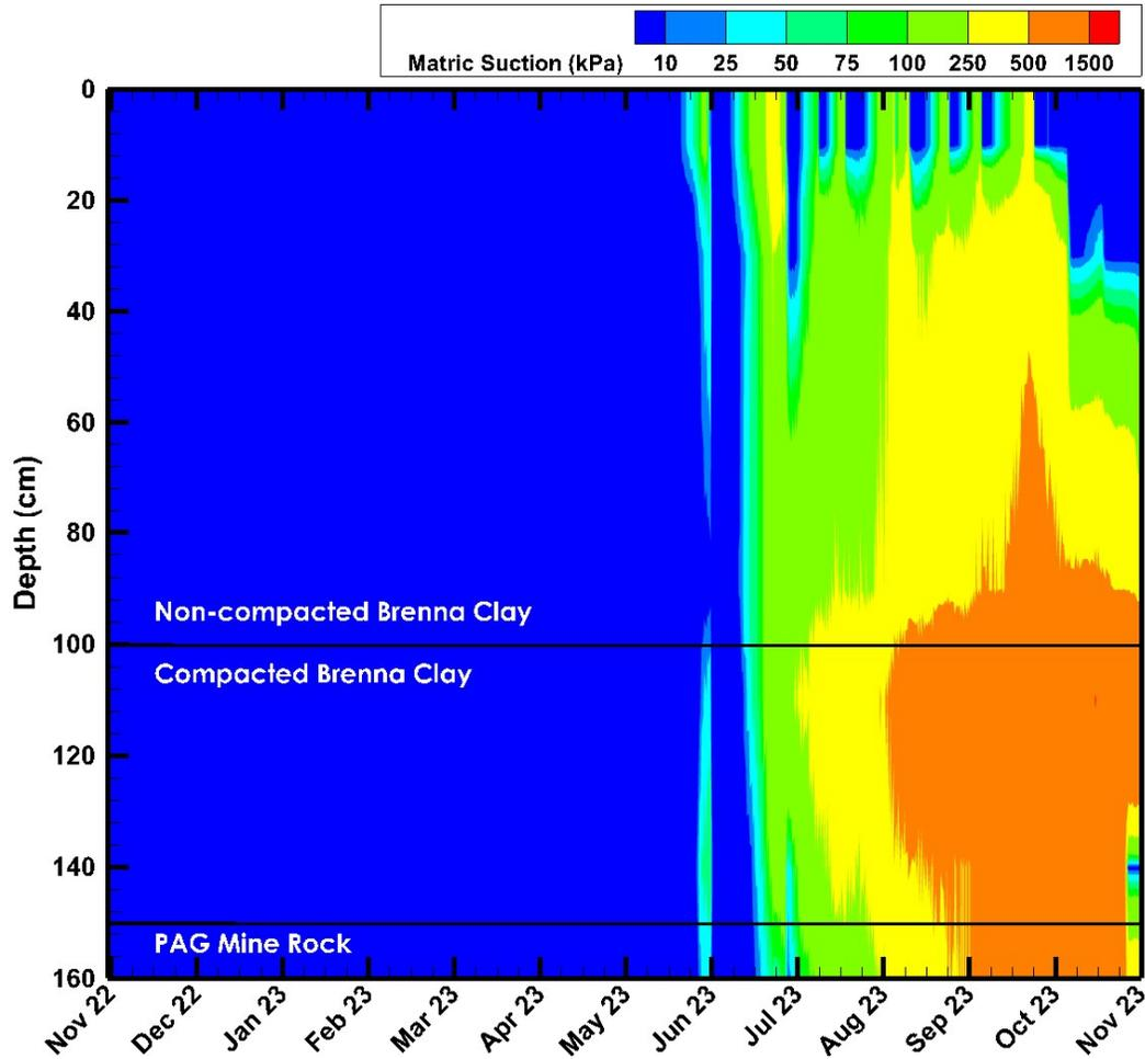
**Figure 3.15: Matric suction measured at the Trial #2 Primary nest.**
