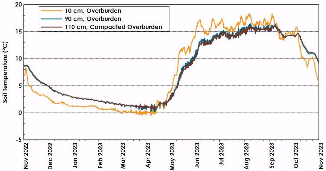
Figure B.12: Temperature profile at the Trial #2 secondary station during the monitoring period.
