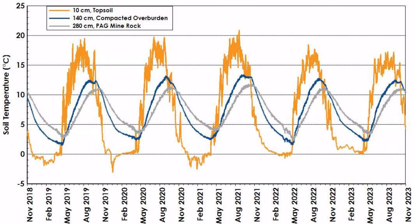
**Figure 3.10: Trial #1 PAG mine rock temperatures since the onset of monitoring.**
