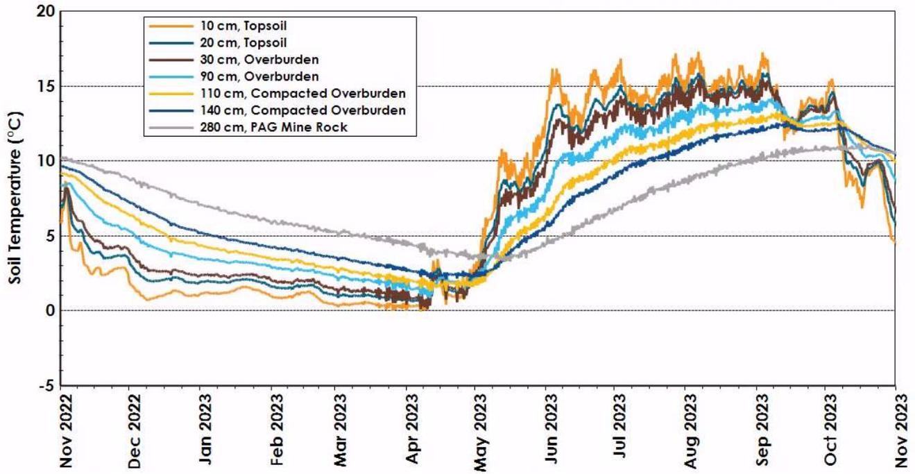
Figure B.9: Temperature profile at the Trial #1 primary station during the monitoring period.
