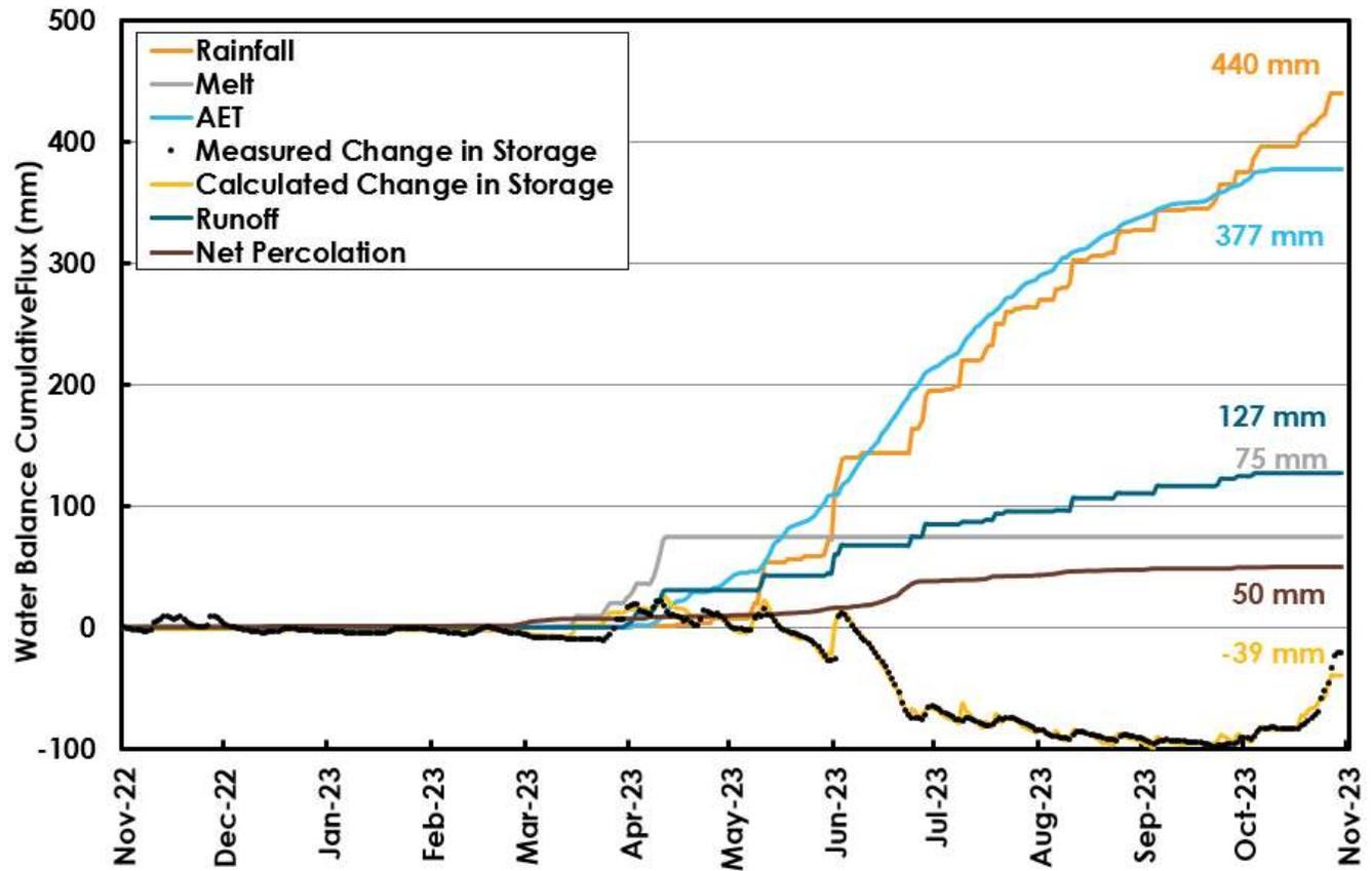
**Figure 3.18: Cumulative water balances flux at Trial #2 for the monitoring period.**
