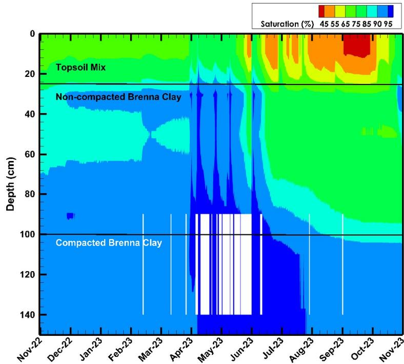
Figure 3.12: Change in degree of saturation at the Trial #1 Primary nest (white areas indicate periods of erroneous data).
