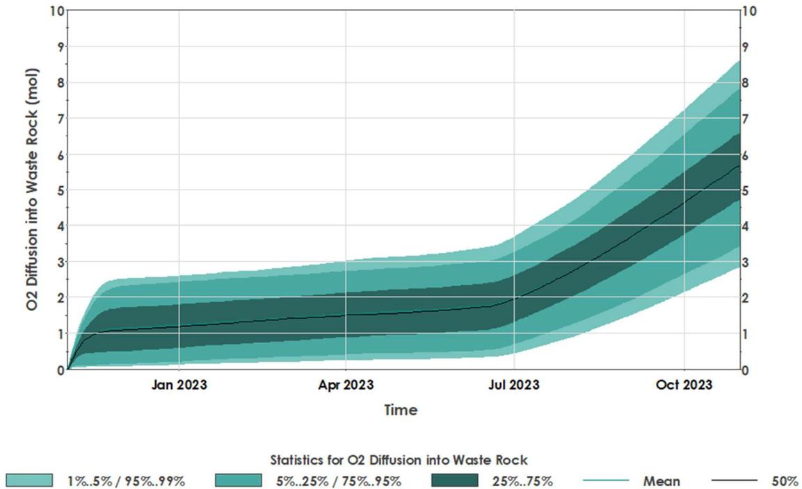
Figure 3.20: Oxygen diffusion simulation through cover materials on Trial #2 over the monitoring period.
