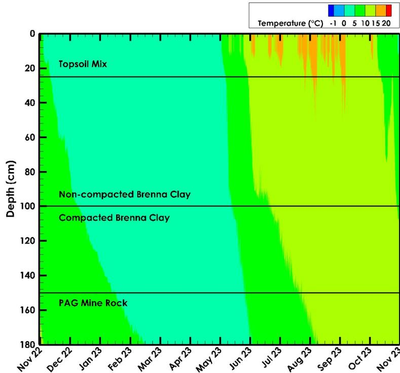
Figure 3.8: Soil temperature profile measured at the Trial #1 Primary nest during the monitoring period.
