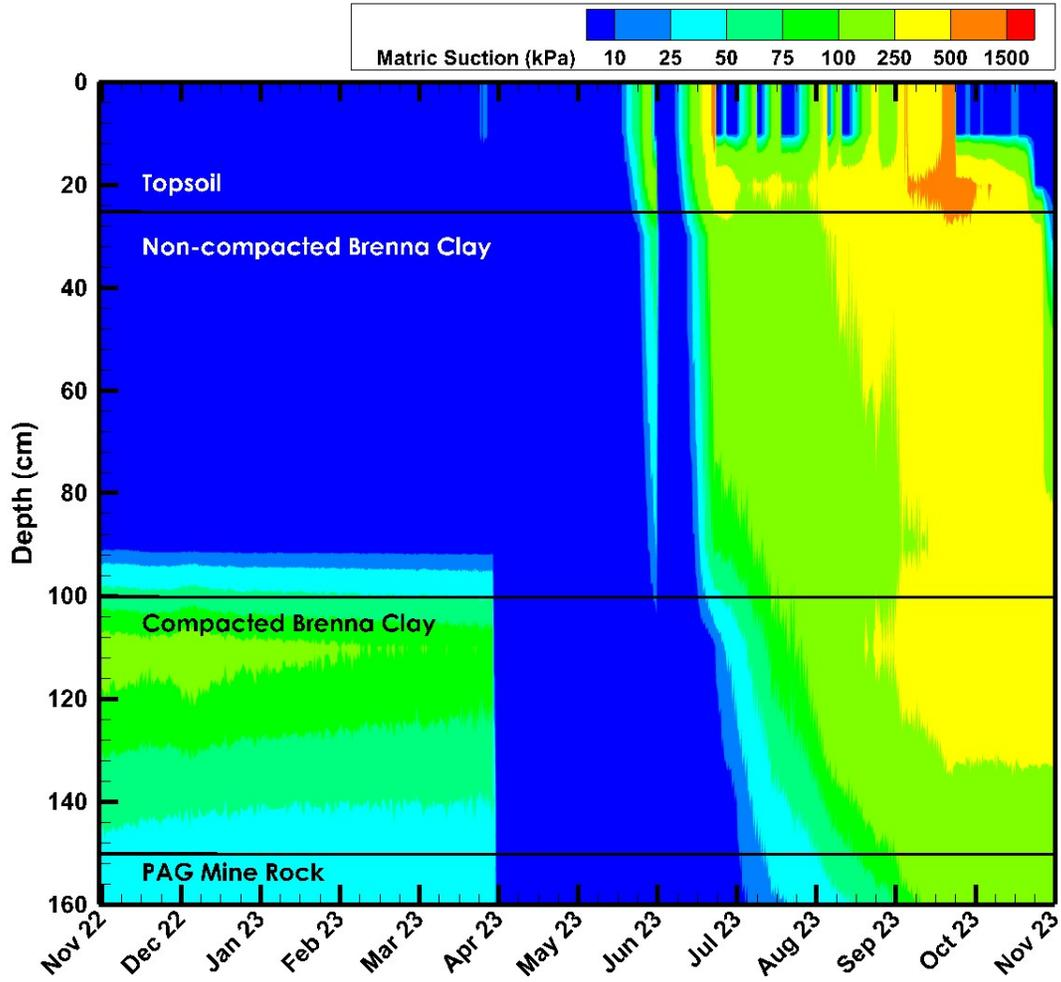
Figure 3.14: Matric suction measured at the Trial #1 Primary nest.
