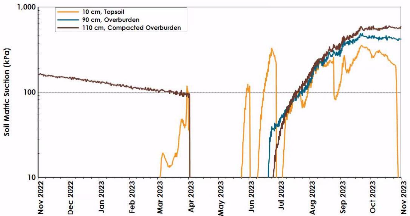
Figure B.6: Suction profile at the Trial #1 secondary station during the monitoring period.
