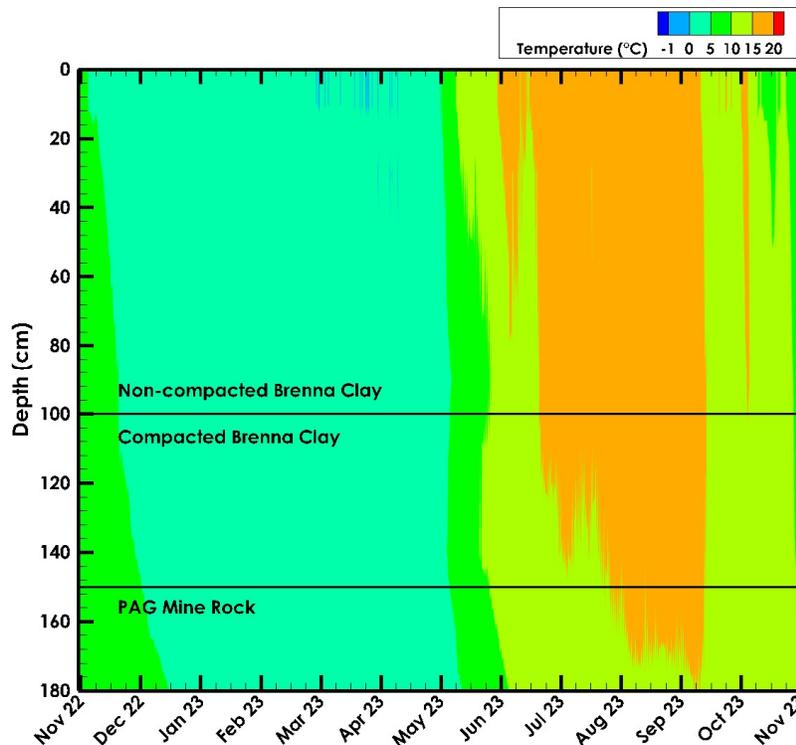
Figure 3.9: Soil temperature profile measured at the Trial #2 Primary nest during the monitoring period.
