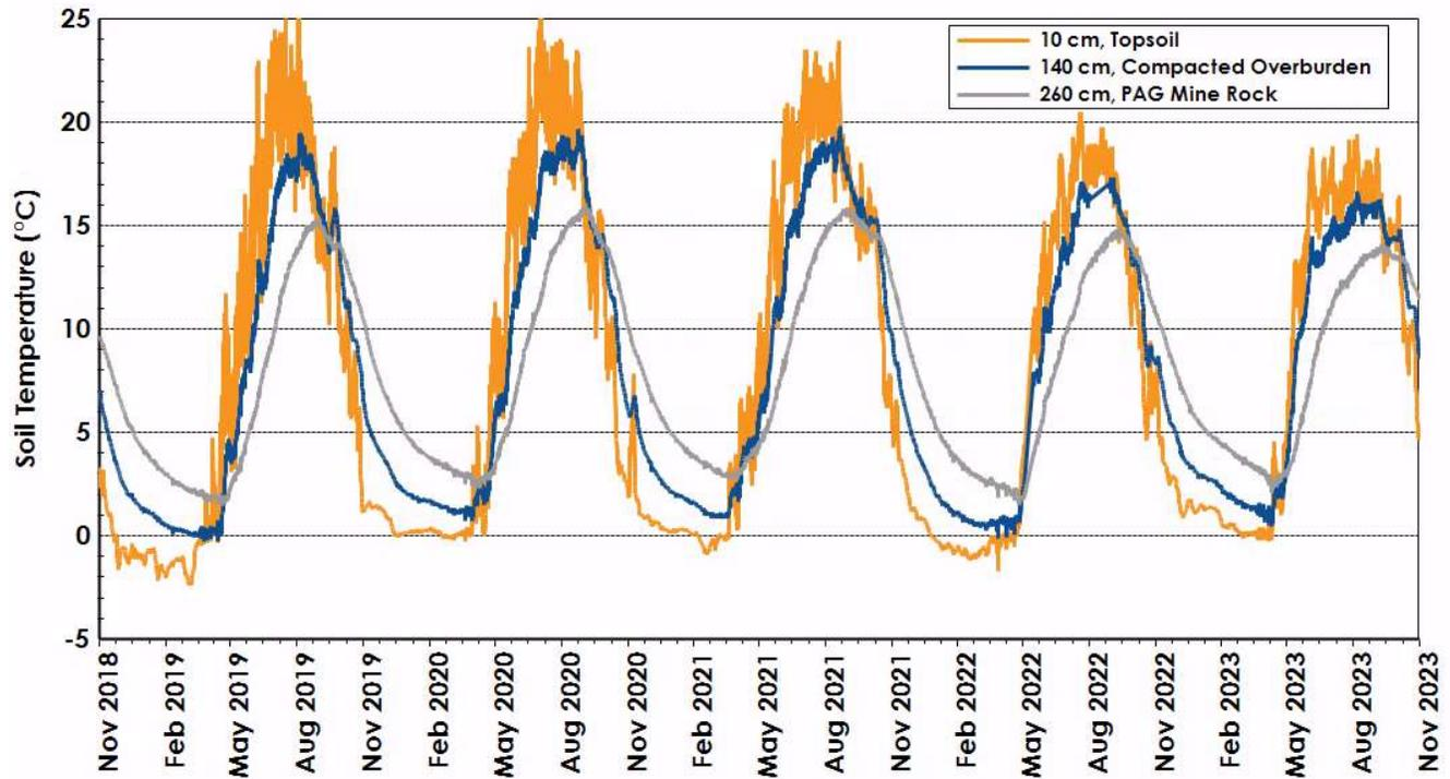
Figure 3.11: Trial #2 PAG mine rock temperatures since the onset of monitoring.
