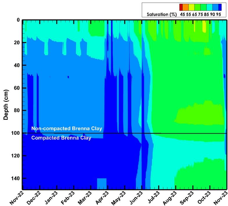
Figure 3.13: Change in degree of saturation at the Trial #2 Primary nest.
