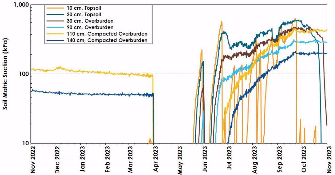
Figure B.5: Suction profile at the Trial #1 primary station during the monitoring period.
