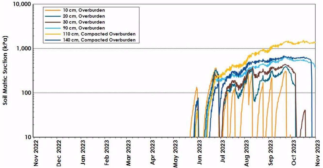
Figure B.7: Suction profile at the Trial #2 primary station during the monitoring period.
