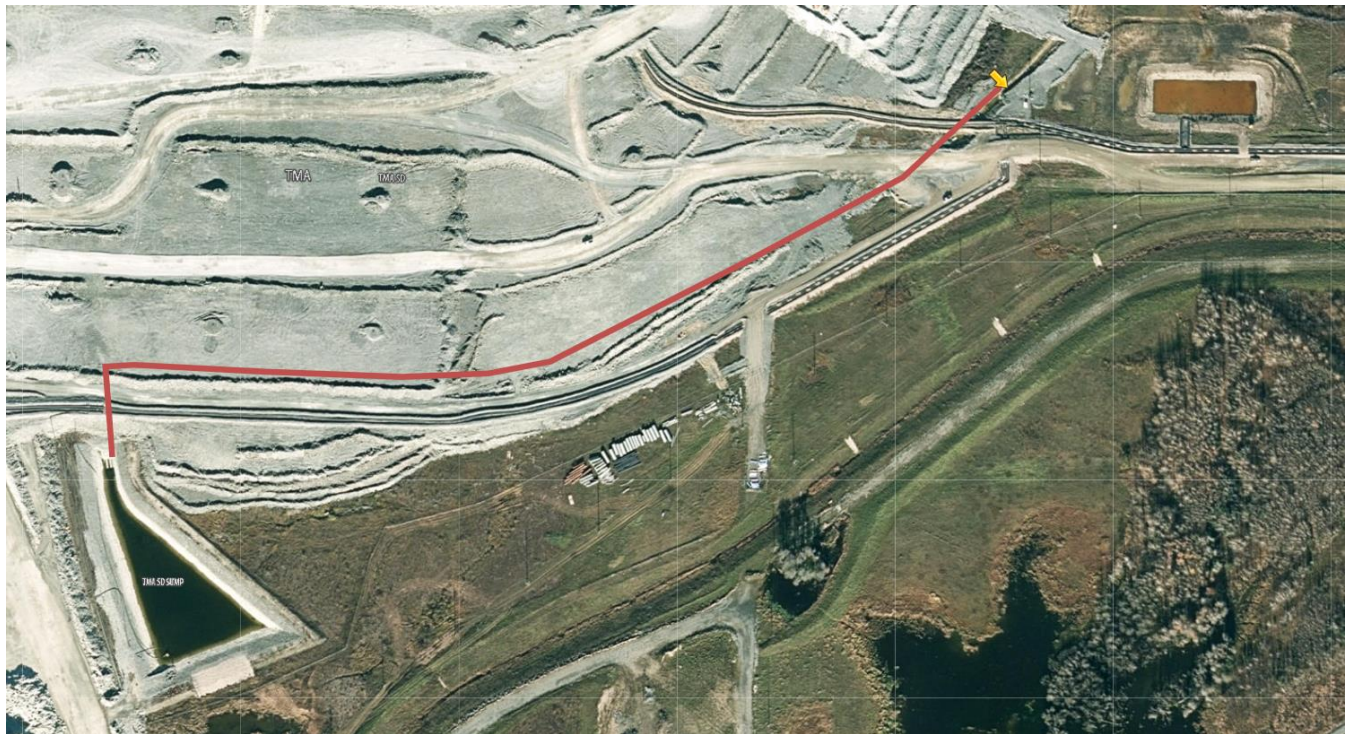
Figure 5 Red line delineates approximate path of South Dam seepage collection ditch French drain. Yellow arrow delineates approximate discharge location of dewatering pump.
