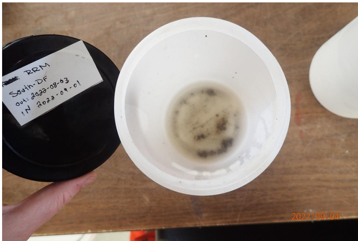
Figure 1: August 2022 South Air Quality Station dustfall canister before shipment to certified laboratory.
