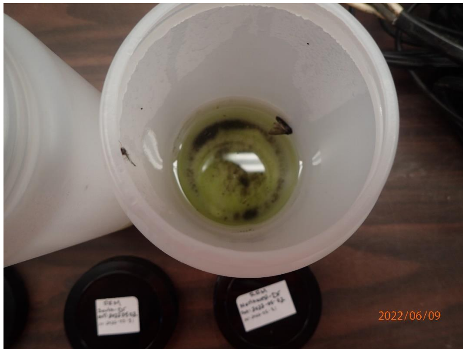
Figure 3 shows May 2022 Northwest Air Quality Station dustfall canister before shipment to certified laboratory.
