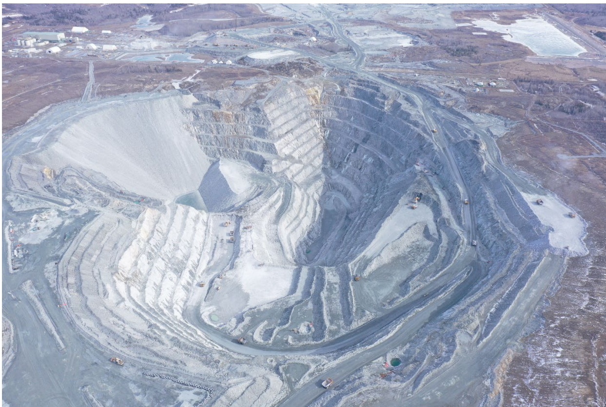
Figure 5. View of the Rainy River pit, looking East. Phase 4 at the bottom of the photo, Phase 3 in the middle, and North Lobe In-Pit Dump on the left. February 22, 2023
