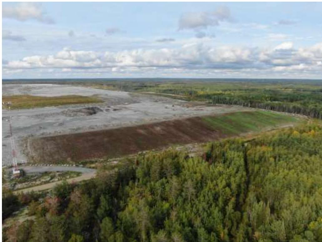
Figure 19. Hydroseed taking on the Southeast EMRS slope (Sept 9, 2021).
