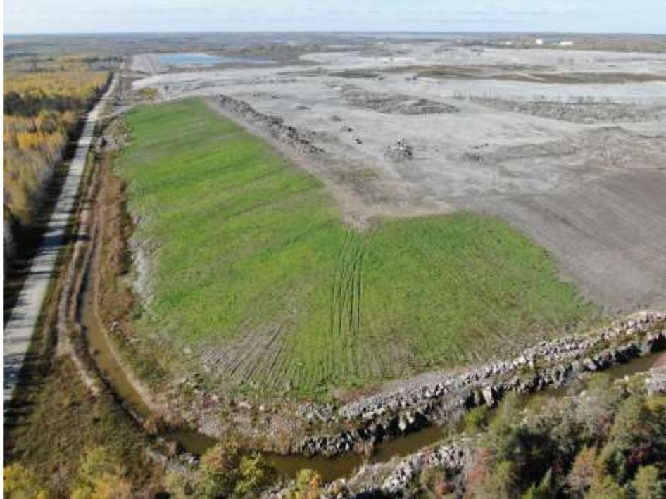
Figure 20. Hydroseed progression on the Southeast EMRS slope (Oct 12, 2021).
