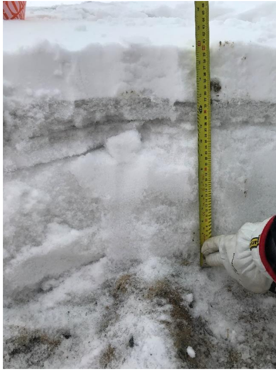
Photo A.1: Snow pack showing snowy facets and layering indicating periods of melting.
