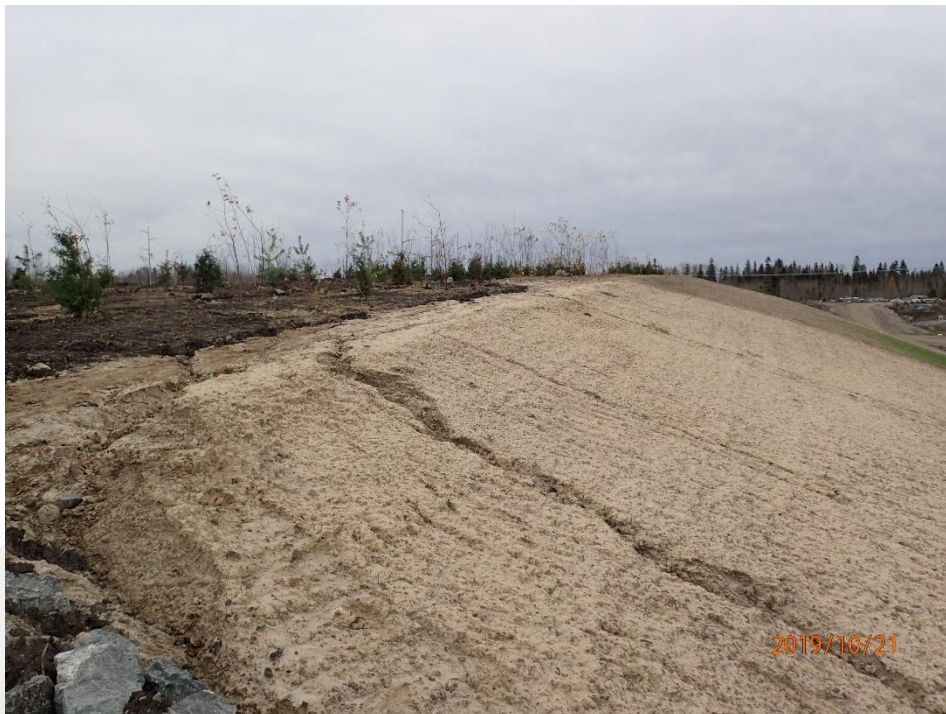
Figure 15: Rill erosion on unseeded control plot.
