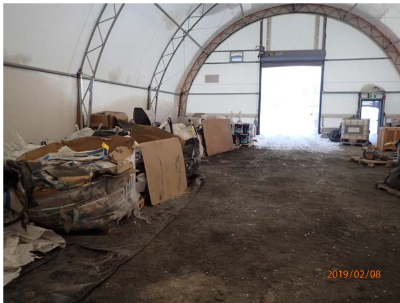
Figure 3: Cleaned up copper sulfate spill inside the covered chemical cold storage building east of the Mill. Damaged totes placed on fold out spill containment.
