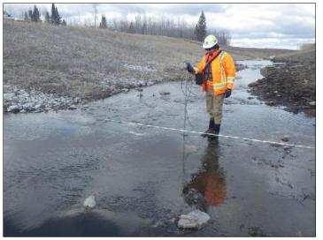
CSS-5 conducting flow monitoring in riffle at outlet (April 26, 2018)
