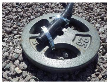
Level logger sensor attached to weight, pre-install (April 24, 2018)
