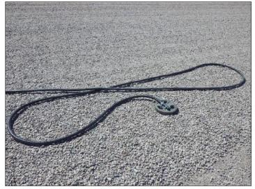
Level logger sensor and cable/tube, pre-install (April 24, 2018)
