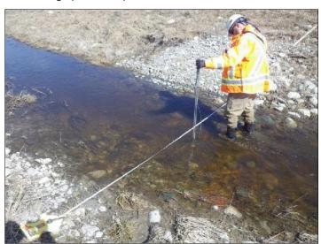
CSS-1 conducting flow monitoring in riffle (April 24, 2018)
