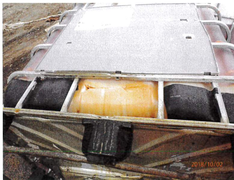
Figure 1 shows Telehandler puncture in the tote of gear oil.
