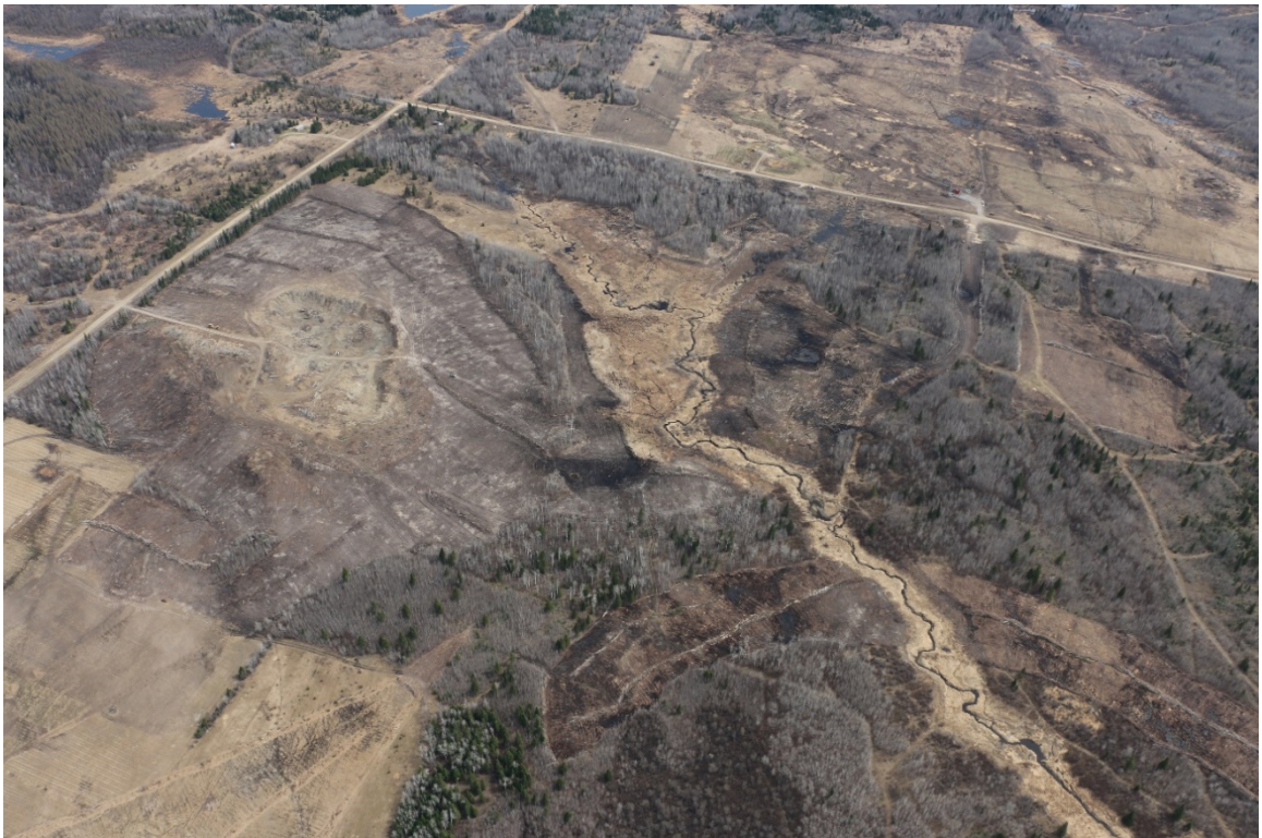
Roen Pit, West Creek Pond, organics and plant site in background showing mulched piles, clearing boundaries and mineral soil protection through vegetation retention
